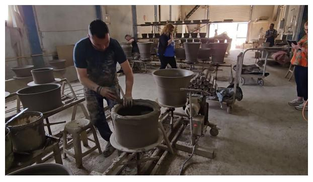
Many of the pots and jars are so large that they are made in distinct stages, with each preceding stage being allowed to dry over night before new clay is added and the next stage formed, sometimes over many days to achieve the larger pots.
