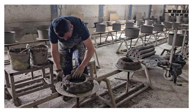
The prepared clay is then formed into cylinders which the potter begins to shape on a potter's wheel. Often, to achieve perfection, the wheel is still turned by hand as can be seen in our video.
