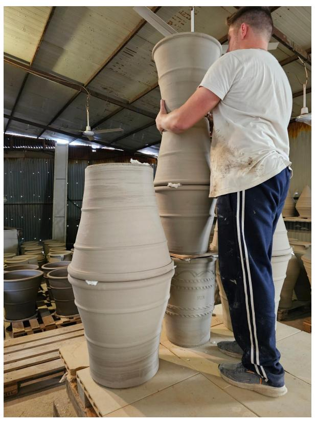
Pots are stacked on giant pallets before being slid into a gas fired kiln at 1200 degrees C. This is much hotter than kilns in other regions and enables the pots to withstand extremes of hot and cold without cracking.
